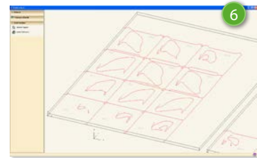
Setting of range and machine code generation that will control the cutting machine
